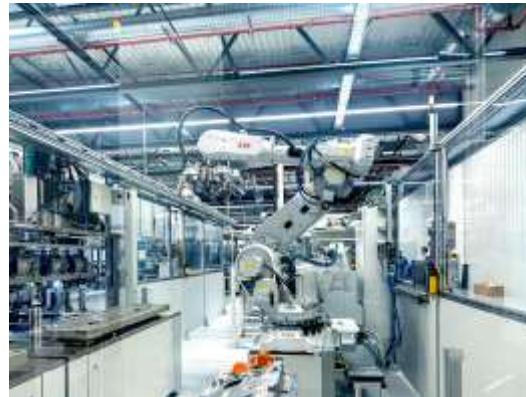
Assembly of Battery Management Controller (BMC) for electric cars with ABB robots.
