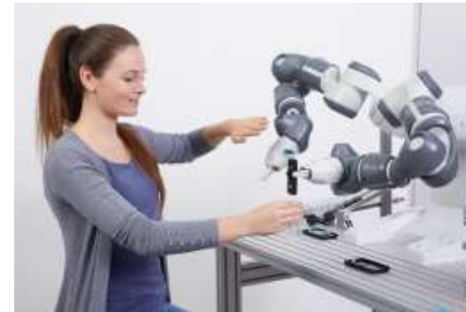
Human robot collaboration with ABB Yumi
