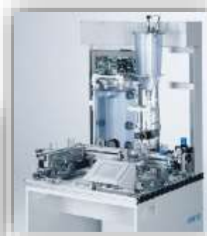
Stations: Filtration, Mixing, Reactor, Bottling closed loop control / process technology
